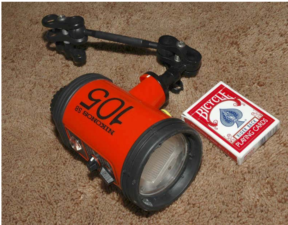
Nikon SB105 "small" strobe – 4 AA batteries
