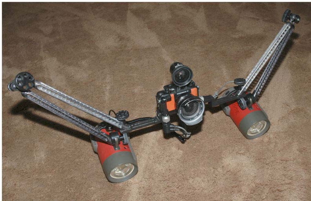
Nikonos V, 15mm lens, SB104 strobes in folded "carrying" position
