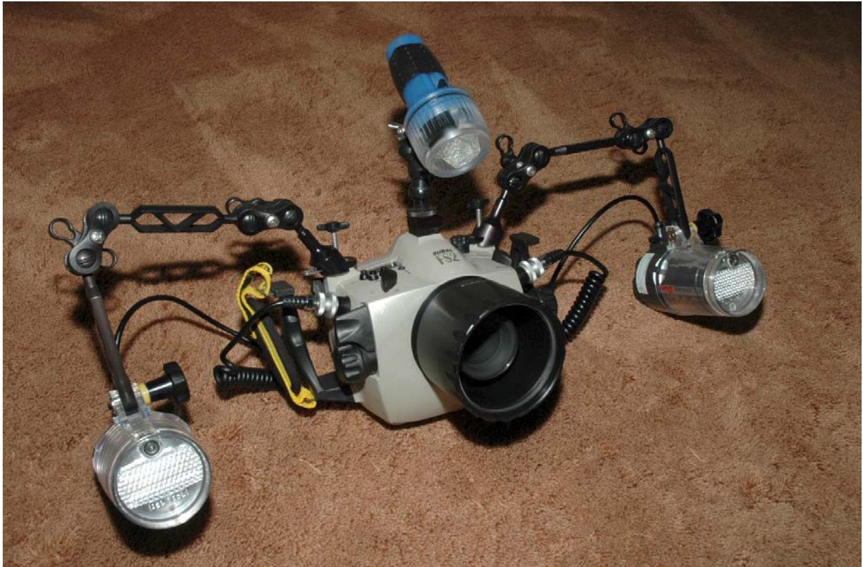
Subal housing, Fuji S2 Pro inside with Nikon 60mm lens, 2 Sea and Sea YS-90DX strobes, ready to hit the water
